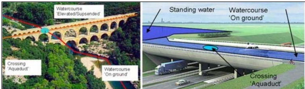
Figure 4 - Aquaduct with two watercourses crossing each other (source: WWW.lesstrainer.nl) and aquaduct crossing a road (water still on ground level)- Extrait de la Spécification Inspire : « D2.8.1.8 Data Specification on Hydrography – Technical Guidelines »
